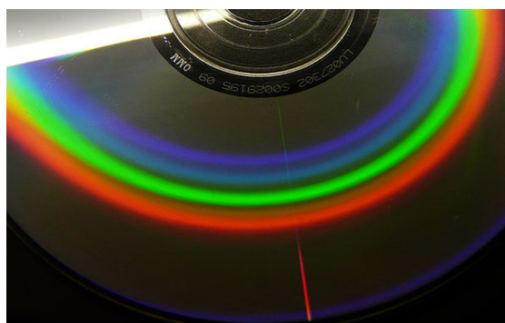
Light from a fluorescent tube lamp reflected by a CD shows the individual bands of color.
