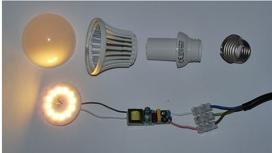
Disassembled LED-light bulb with driver circuit board and Edison screw
