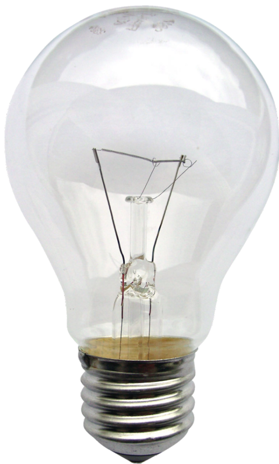
A 230-volt incandescent light bulb, with a 'medium' sized E27 (Edison 27 mm) male screw base. The filament is visible as the horizontal line between the vertical supply wires.
