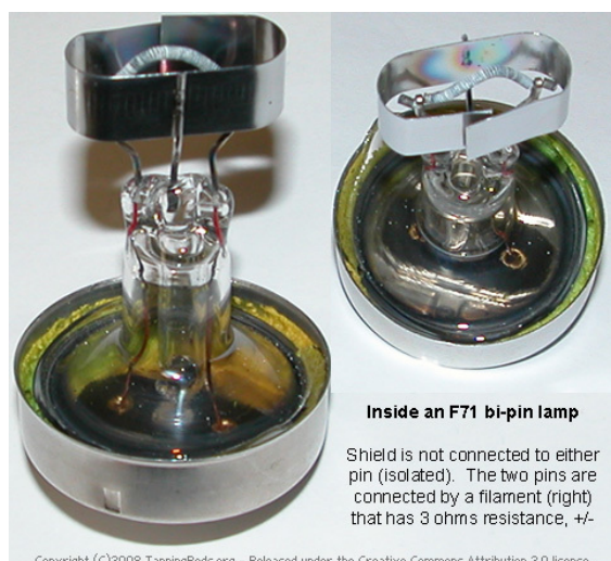
Inside the lamp end of a preheat bi-pin lamp. In this lamp the filament is surrounded by an oblong metal cathode shield, which helps reduce lamp end darkening. [2]
