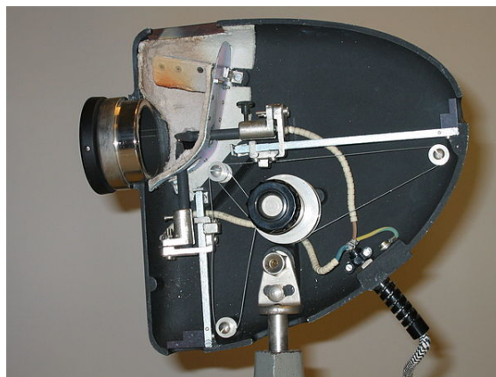
A carbon arc lamp, cover removed, on the point of ignition. This model requires manual adjustment of the electrodes
