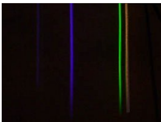
Line spectrum of mercury vapor. The blue-green tint of mercury vapor lamps is caused by the strong violet and green lines.
