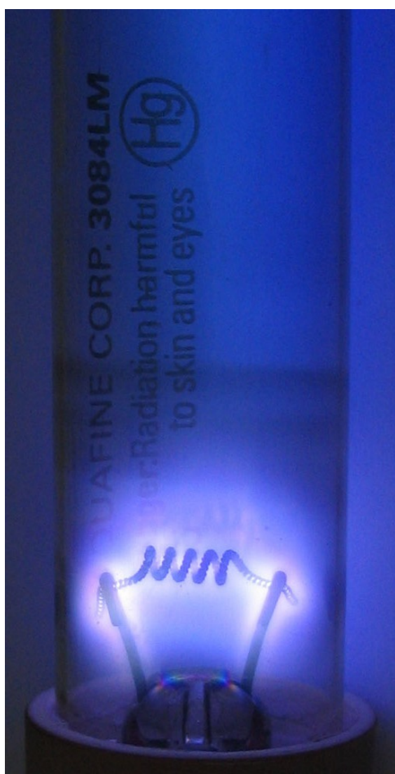
Germicidal lamps are simple low-pressure mercury vapor discharges in a fused quartz envelope.
