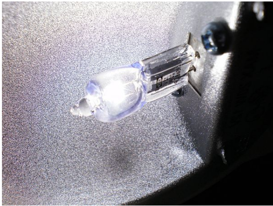
A halogen lamp operating in its fitting with the protecting glass removed
