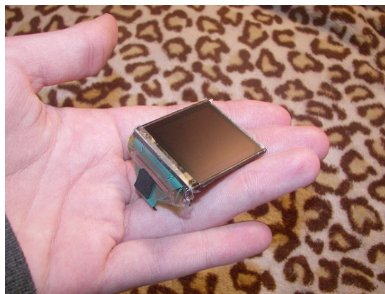
A 3.8 cm (1.5 in) OLED display from a Creative ZEN V media player
