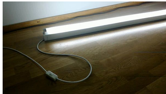
Fluorescent lamp with an electronic ballast.
