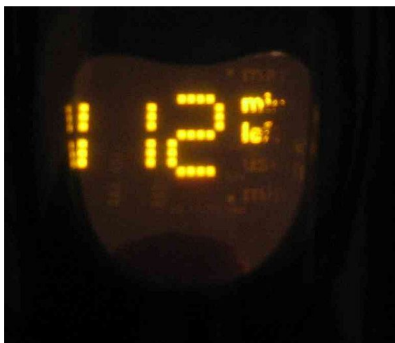
LEP (light emitting polymer) display showing partial failure
