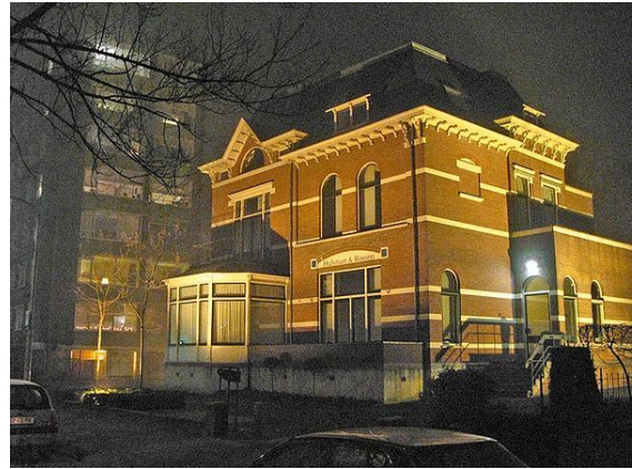
Office building illuminated by high-pressure sodium lamps. Note the lamps shining upward, of which much light goes into the sky and neighboring apartment blocks, causing light pollution.
