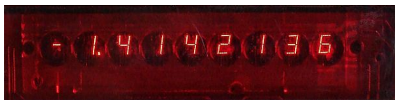
LED display of a TI-30 scientific calculator (ca. 1978), which uses plastic lenses to increase the visible digit size
