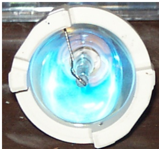
An Osram 100 W xenon/mercury short-arc lamp in reflector
