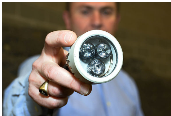
LED to be used for miners, to increase visibility inside mines.
