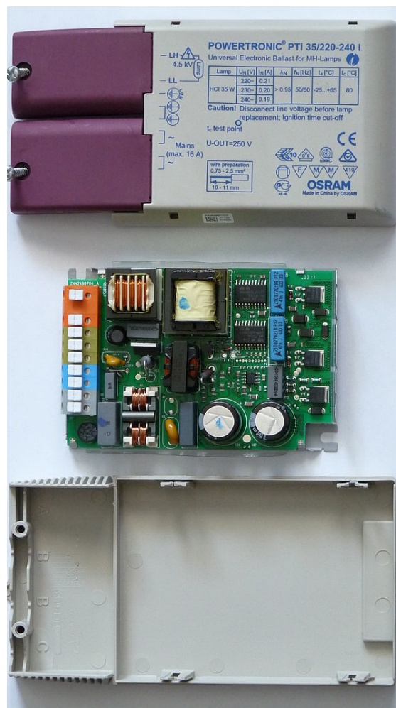
Electronic ballast for 35W metal halide light bulbs
