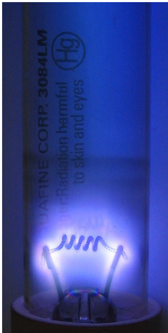
The unfiltered ultraviolet glow of a germicidal lamp is produced by a low pressure mercury vapor discharge (identical to that in a fluorescent lamp) in an uncoated fused quartz envelope.
