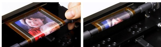
Demonstration of a 4.1" prototype flexible display from Sony
