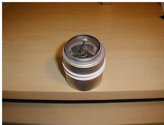
A Cermax 2 kW xenon lamp from a video projector. A pair of heatsinks are clamped on the two metal bands around the perimeter, which also double to supply power to the lamp
