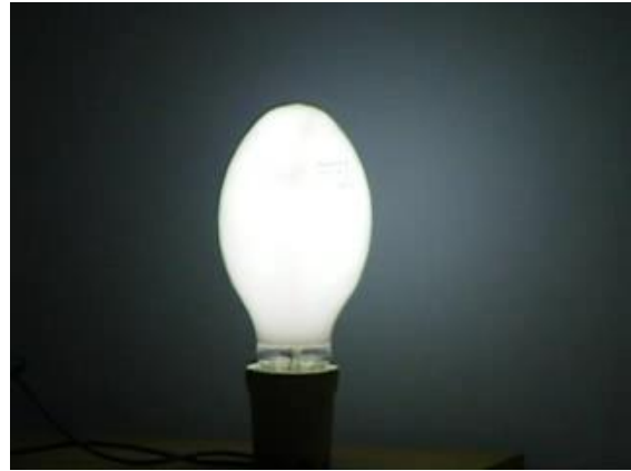
Warm-up of a color corrected 80 W high-pressure mercury vapor lamp to half brightness
