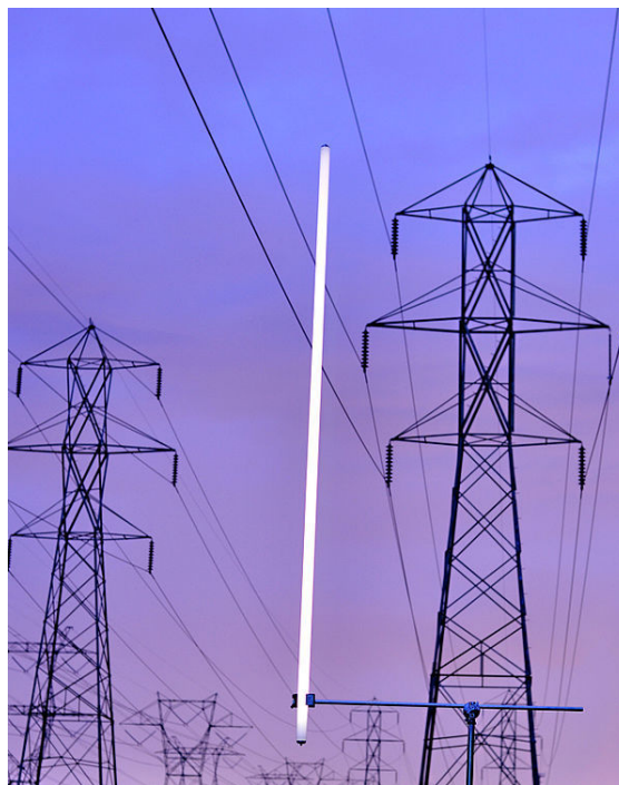
Capacitive coupling with high-voltage power lines can light a lamp continuously at low intensity.
